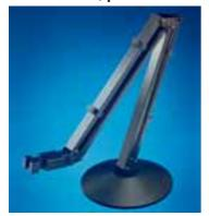
Electrode arm moves smoothly in almost any direction, holding up to 4 electrodes + 1 temperature sensor safely and securely in selected positions. Fingertip control raises, lowers, and pivots the holder. The arm articulates at three points while maintaining electrodes in a vertical position.
